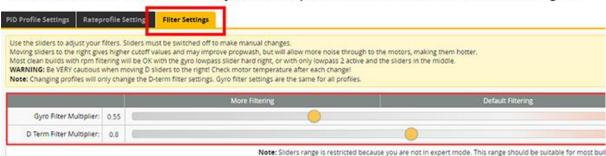
2. Adjust the filter setting as shown in the figure. The value in the first row is 0.55, and the value in the second row is 0.8 (sliding slider)
