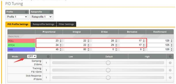
1. Set the arrow to "off" and then adjust the PID parameters with reference to the above figure.
